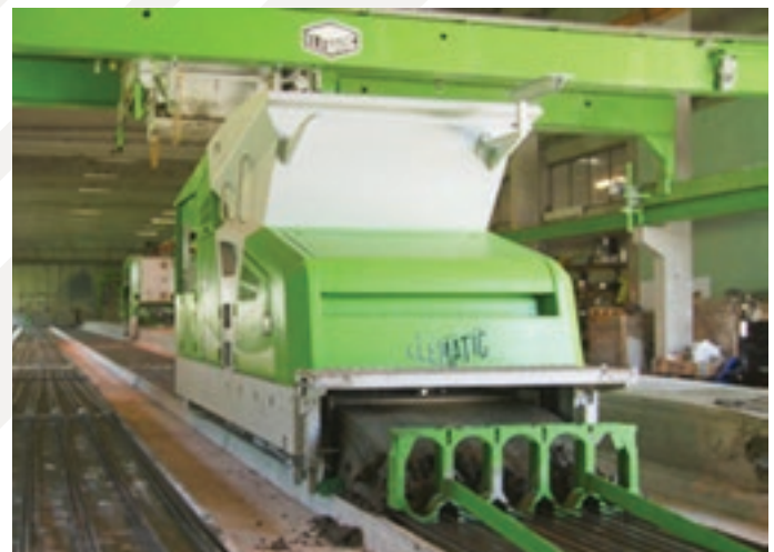
Extruder machine for production of hollow core slabs
